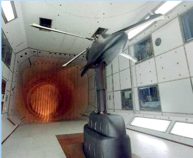
Rotor test rig and experimental rotor in QinetiQ 5 metre wind tunnel HC(AG) on "Validation of rotor blade / hub load synthesis techniques"
